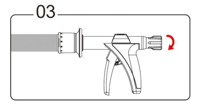
Insert the pull road into stapler, turn right the rotating knob smooth tightly to check the indicator in the window.
