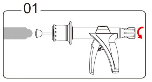
Turn left the rotating knob, pull out the penis cabin and staple cap.
