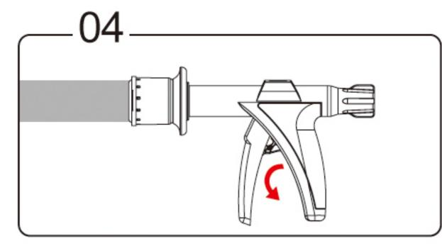
Pull down the safety clasp and ready for firing.
